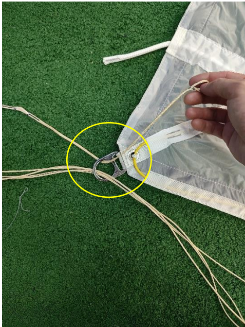
Figure 2.7 Left steering line through left rear slider ring.
