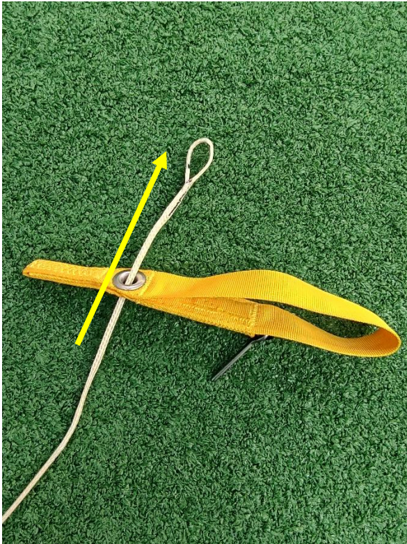
Figure 2.9 Route steering line from bottom of the toggle.
