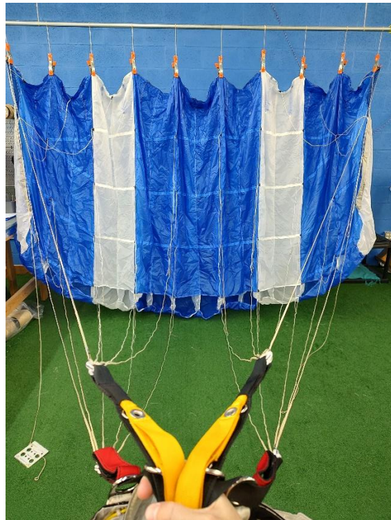
Figure 2.4 Suspension lines attached to risers.
