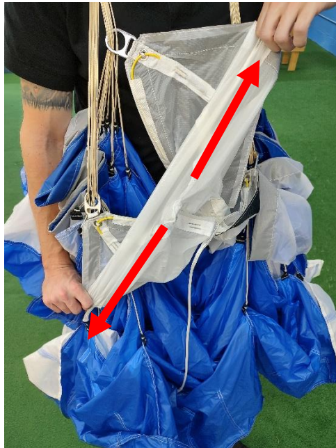
Figure 2.15 Pull collapse cable back into the slider.
