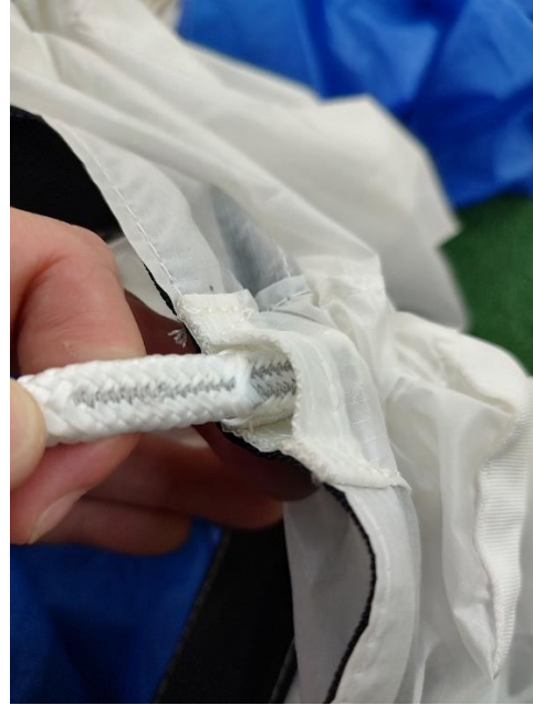
Figure 2.14 Insert the locking tab into the channel.
