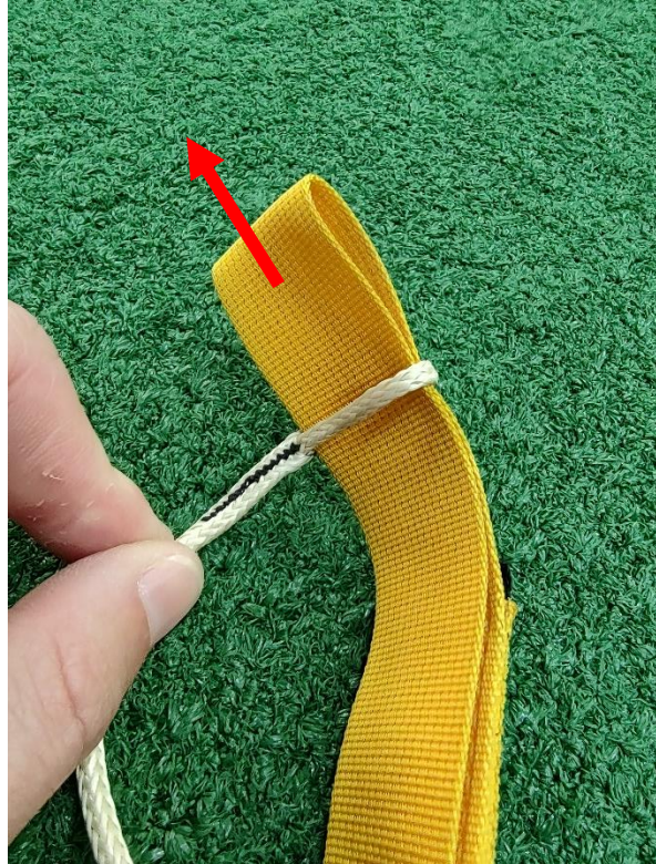
Figure 2.10 Route the handle of the toggle through the loop end of the steering line.
