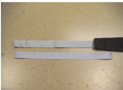
6. Cut a piece of TYPE 12 Webbing as shown. Cut the Webbing 6" longer than Leg Pad overlap.
